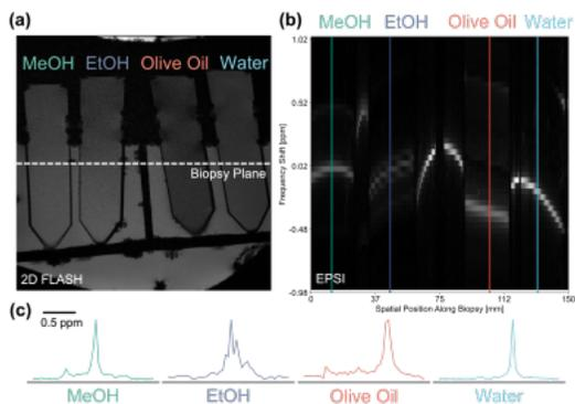
EPSI spectroscopic analysis of a phantom containing four chemical samples: methanol (MeOH), ethanol (EtOH), olive oil, and water. (a) Reference 2-D FLASH scan of the phantom setup indicating the virtual biopsy readout axis. (b) EPSI virtual biopsy  $T_2$ -weighted spectrum. (c) Plotting the 1-D MR spectra at the four indicated locations demonstrate the expected peaks for each of the imaged compounds.
