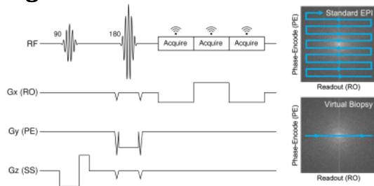
(Left) MR pulse sequence diagram for our EPSI-like virtual biopsy sequence. (Right) Visual illustration of our virtual biopsy *k*-space trajectory compared to that of typical EPI imaging approaches.
